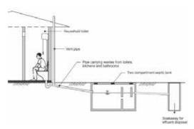
• Flush to piped sewer system: A system of sewer pipes designed to collect human excreta and wastewater and remove them from the household environment. Sewerage systems consist of facilities for collecting, pumping, treating, and disposing of human excreta and wastewater.
