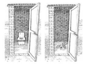
• Pit latrine without slab/open pit: A latrine without a squatting slab, platform, or seat. An open pit is a rudimentary hole in the ground where excreta is collected.
