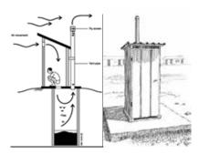
• Pit latrine with slab: A latrine that uses a hole in the ground for excreta collection and has a squatting slab, platform, or seat (made of concrete, steel, or wood to allow standing with ease) that is firmly supported on all sides, easy to clean, and raised above the surrounding ground level to prevent surface water from entering the pit.
