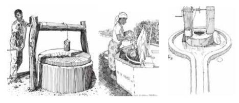
• Unprotected dug well: A dug well for which one or both of the following conditions is true: (1) the well is not protected from runoff water; or (2) the well is not protected from bird droppings and animals. If at least one of these conditions is true, the well is unprotected.
