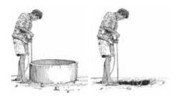
• **Protected spring:** A spring typically protected from runoff, bird droppings, and animals by a spring box, which is constructed of brick, masonry, or concrete and is built around the spring so that water flows directly out of the box into a pipe or cistern without being exposed to outside pollution.
