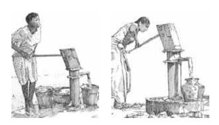
• **Protected dug well:** A dug well that is protected from runoff water by a well lining or casing that is raised above ground level and a platform that diverts spilled water away from the well. A protected dug well is also covered, so that bird droppings and animals cannot fall into the well. Both conditions must be observed for a dug well to be considered as protected.
